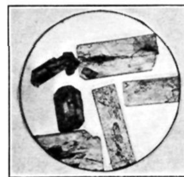
Fig. 4.—Photomicrograph (12 X) of monoclinic Na 3 PO 4 formed at 250°.
